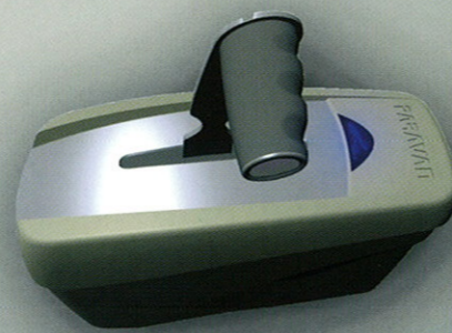
Electronic-digital accelerator and brake system also available with armrest
